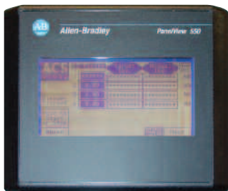
Programmable entry screens for all three recipe modes (up to six components)
